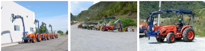
STI supplied for four trains consisting of Shot-Tech Robotic Arm, Tractor, Accelerator Pump and Shotcrete Pump
