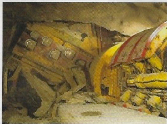
The Wirth TBE undercutting system comprises cutter discs mounted on six radial arms, which are inclined backwards from the centre of the tunnel
